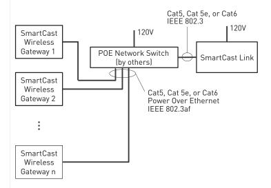
SmartCast® Wireless Gateway with Wi-Fi (CSC-GW-CWC-W)
