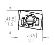
Note: For use with a standard 1/2" EMT knockout.
