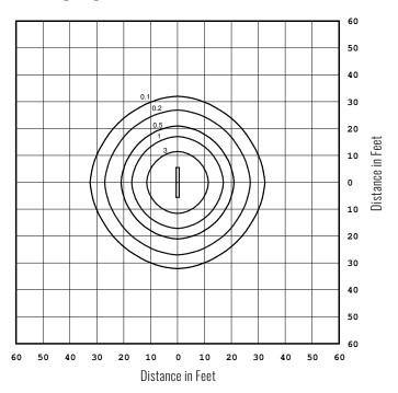
**Note**: All published photometric testing performed to IES LM-79 standards. Fixture photometry was completed on a single representative fixture. Foot candle levels are noted inside graph. **Visit e-conolight.com for the latest EPA data.**
