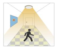
When motion is detected, the sensor will switch on the light to 100% brighteness.
