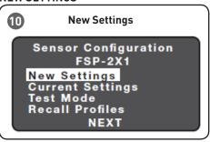
New Settings allow you to select the different sensor parameters such as: High/Low Mode, Time Delay, Cut Off, Sensitivity, Setpoint, Ramp/Fade rates and Photocell. See
